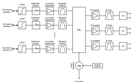
Fig. 2. SPACEBEAM receiver high level block diagram.
