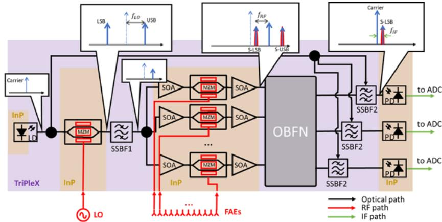
Fig. 3. SPACEBEAM PIC architecture.
