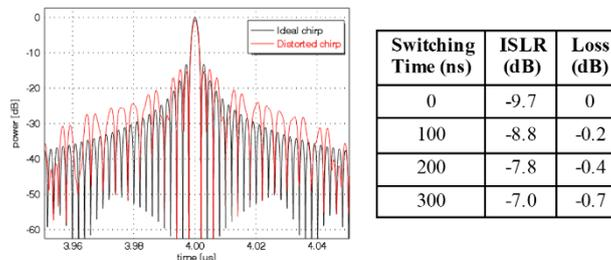
Fig. 4. Impact on switching of beamforming weights on the IRF.
