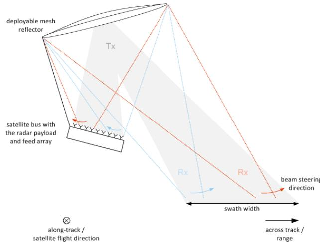
Fig. 1. Illustration of scan-on-receive (SCORE) imaging mode.
